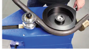
PIPE / STRUCTURAL BENDING
