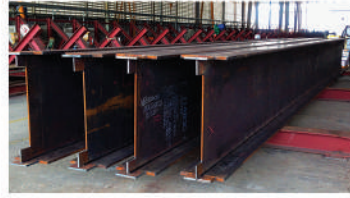
BUILD UP HEAVY BEAMS
